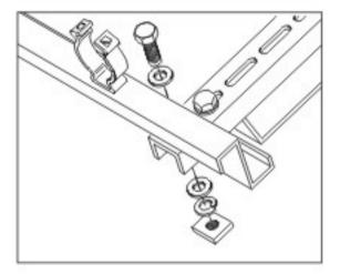
Install the bottom support on the third hole of the vertical support; fasten screw to avoid the bottom support slipping.
