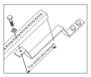
Install vertical supports on the roof hooks as picture shows, keeping the same extended length on top and bottom of the supports and install the bolts on the long hole according to drawing to avoid vertical supports slip. Then only fix screws slightly. (Continue to item 3)
