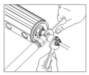
As picture shows, tighten the thermowell. Check and adjust the sensor in order to make it work well.
