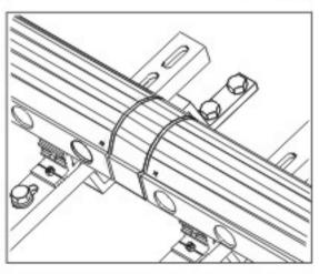
Fasten the support of header box with the screw to clamp the connection cuff.
