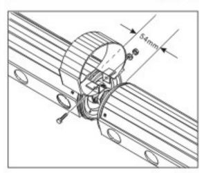
Insert the insulation material in the space, and on which cover the connection cuff.
