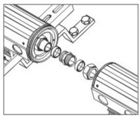
Connecting two header boxes with two-end fitting in series or according to the advanced design. To keep granularity of 54mm between the two header boxes.
