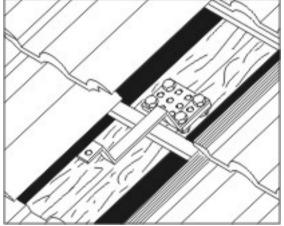
If necessary use the attached perforated plates to achieve the above measure (see data in item 1). The roof hooks must be mounted vertically and horizontally in alignment.
