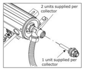
Install thermowell, which is for sensor, on the outlet pipe. Smear some heat transmission paste on sensor and insert the sensor into the thermowell.
