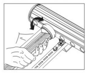
Adjust vacuum tube and keep the selective coating side to face upward.
