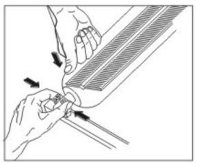
Put the end cap of tube into the clip, if necessary adjust the location of the bottom support. The end of the tube shall rest on the rubber strip of the bottom support. Close clip.
