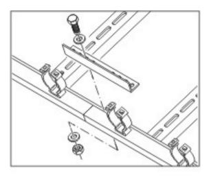
Connect two bottom suppports with L-profile and tighten screws.
