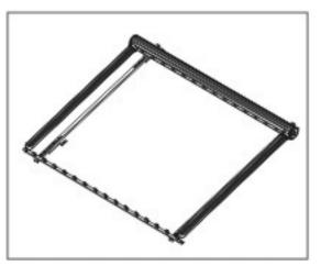
From right to left install the vacuum tubes, keep whole collector in parallel and note that the header box is not exact horizontal, but there is a small slope downwards to inlet.
