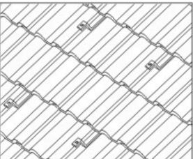
As picture shows, put tiles on the roof hooks, and it must be made water-proofed.
