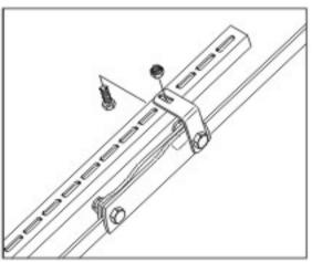
Installing vertical supports on the roof hooks as picture shows, to keep the same stretched length between up and down and then fasten the bolts on the long hole according to the drawing to avoid vertical supports slip. Then only fix screw slightly. (Continue to item 3)
