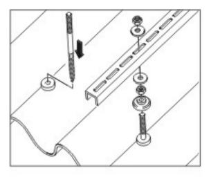
c) Install the roof hook on eternit corrugated roof Install the thread pole on the rafter, and then install vertical support with spacer keeping the same stretched length between up and down. Fasten the bolts on the long hole according to drawing to avoid vertical supports slip. Then only fix screw slightly.
