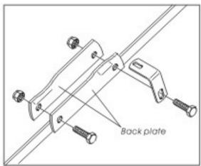
b) Install the roof hook on steel plate roof.
